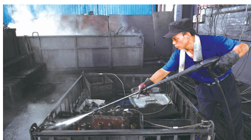
“炖煮”后再对部件进行冲洗,彻底清除污垢
